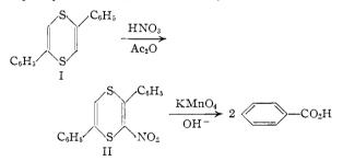
The position of the nitro group was assigned on the basis of potassium permanganate oxidations. Several oxidations were performed and in no experiment was any nitrobenzoic acid found. This observation, along with the isolation of benzoic acid in 67% yield (calculated for 2 moles of acid per mole of II) led to the assignment of structure II for the nitro derivative. The experiments to follow support this assignment of structure.
